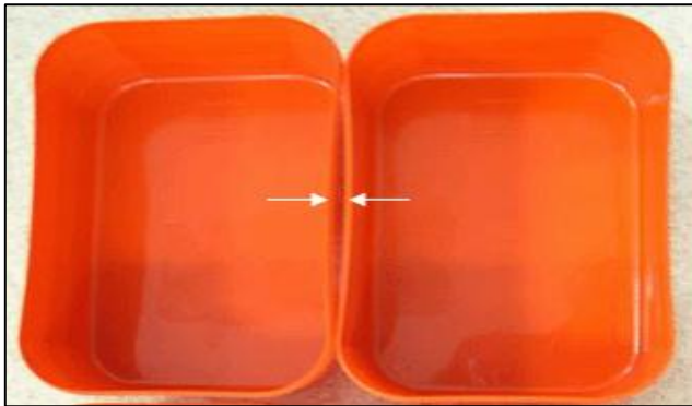
Fig. 3. : Example of product affected by warpage.
